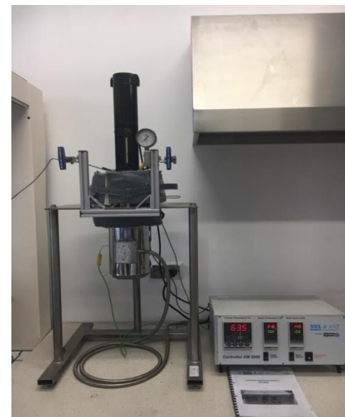
High pressure reactor
